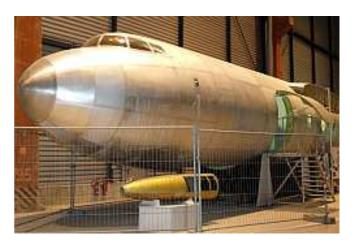
In an adjacent building the group was shown the EADS program for converting passenger transports into freighters. Several Airbus 300 series aircraft were in the process of having their interiors gutted, windows removed and floors strengthened for further service in this important sector of the global aerospace industry.
